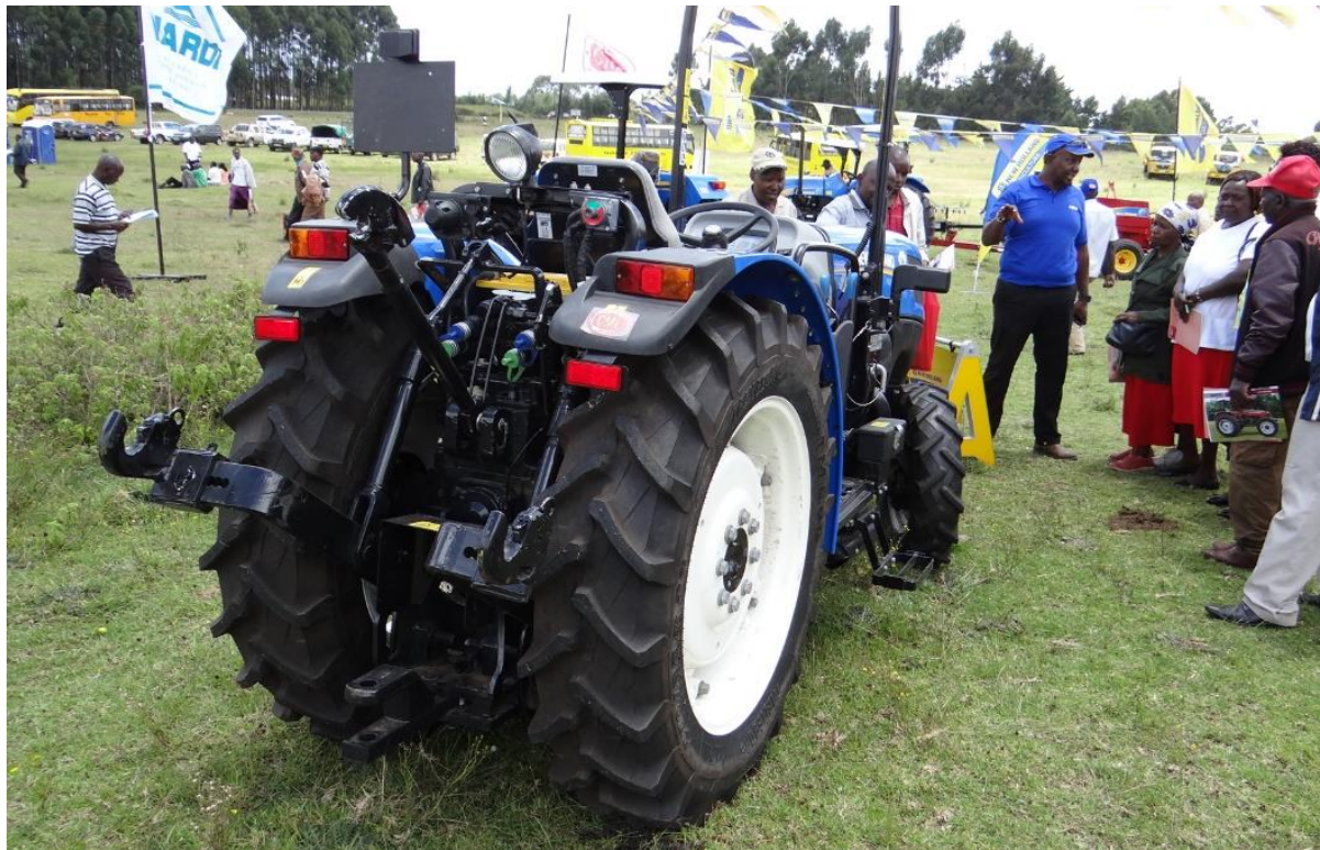
Special narrow wheelbase tractor for working between orchard trees. Special custom-made tractors like this one can be more expensive than a higher power and bigger size tractor.
